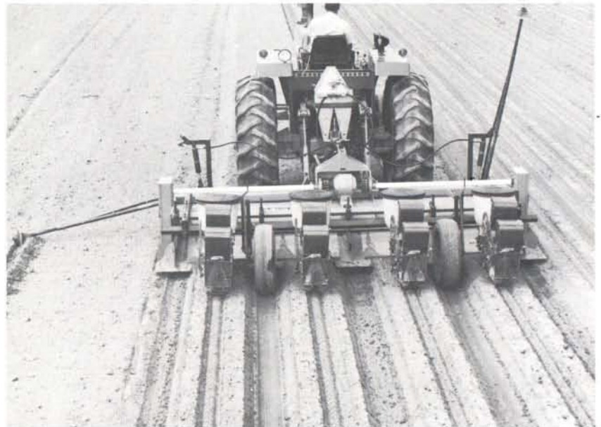
Model No. 80-144 Ferguson Tilrovator featuring Va. P-nut special bed shapers. Bed 3" high and 21" wide on top. Results in firm bed top for seed placement. Other model bed shapers available for bed heights from 2" to 9" and most row spacings.
