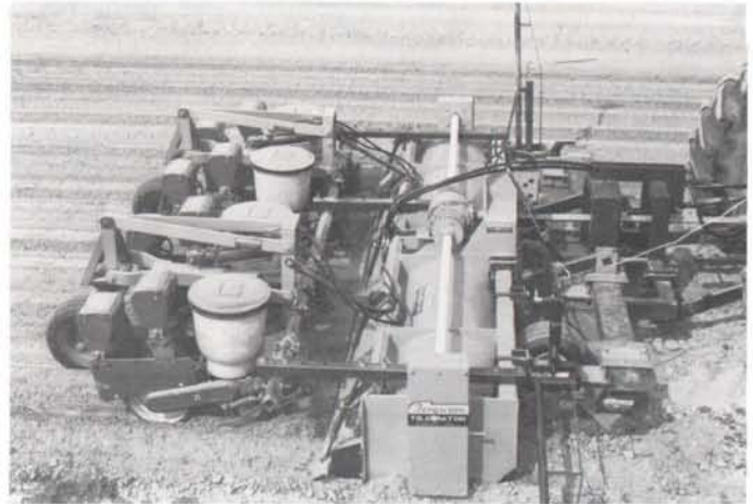
Model No. 80-144 shown adapted to Ferguson row ripper enabling you to under the row sub-soil – til – incorporate and plant in one pass. Also equipped with hydraulic lift assist wheels so that tractors in the 100-115 H.P. range can do this complete job of planting.
