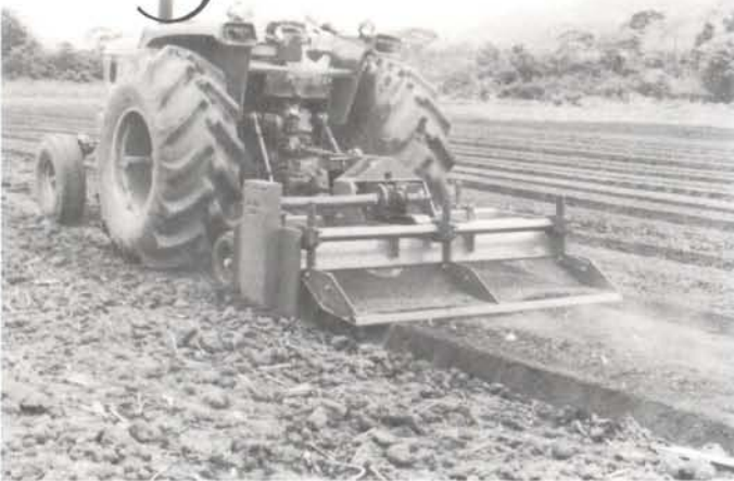
Model 80-80 Ferguson Tilorovator with SW-2-38-7 Bedshaper. P.T.O driven tiller mulches clods while bedshaper (attached to rear frame bar) shapes beds to uniform dimensions: height of bed from 3" to 9". Above photo demonstrates shaping of wide vegetable bed 7" high and 61" across top. Available for most row spacings. Auxiliary bar may be attached to adapt unit planters for once-over planting operation.
