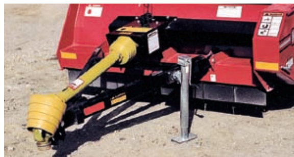
A constant-velocity P.T.O. shaft protects the driveline during turns, reducing wear on drive components.
