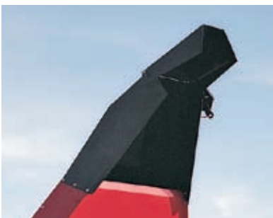
Adjustable discharge spout is controlled from the tractor seat for easy, even loading.
